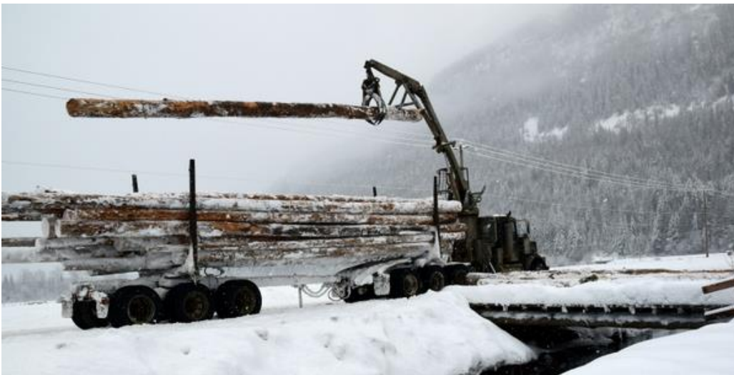
Logs that can be used to support the excavator and to place in the wetlands may be ordered. This load of 45-logs costs $2,500 at Meadow Creek, BC
